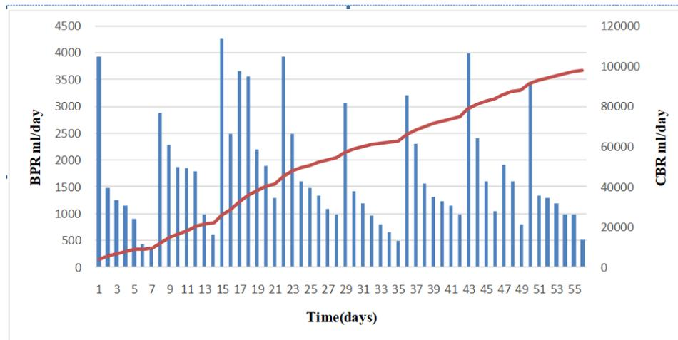
**Figure 1:** Biogas production rate (BPR) and cumulative biogas production (CBP) in the methanogenic reactor in 2-stage co-AD of chicken dung and food waste
