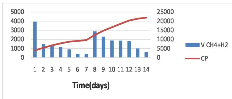
**Figure 2.** Methane and hydrogen production rate and cumulative production (CP) for one cycle of co-AD of substrates in two-stage mode
