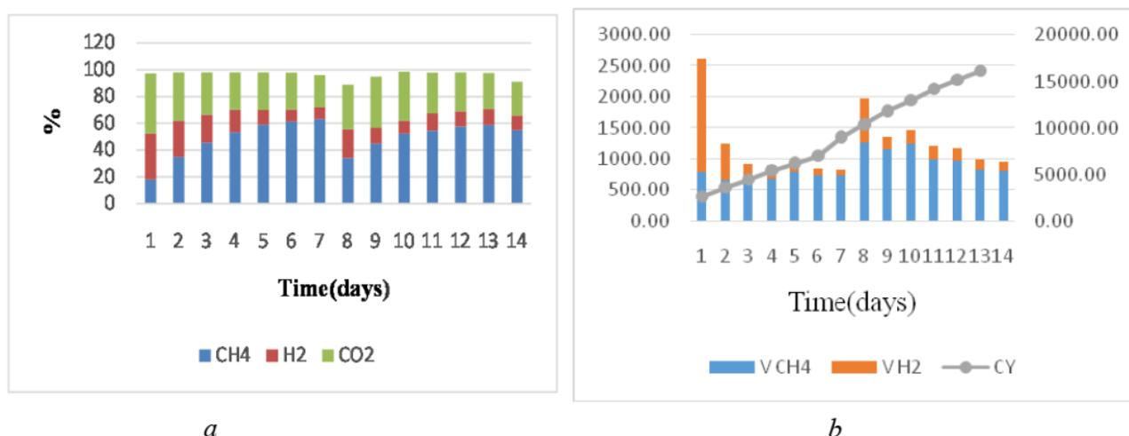
**Figure 3:** Characteristics of **14-day cycle** of anaerobic decomposition of a substrate in a 2-stage set-up: a) Kinetics of methane (CH<sub>4</sub>), carbon dioxide (CO<sub>2</sub>), hydrogen (H<sub>2</sub>) production during co-AD and b) Volumes of methane and hydrogen with a cumulative yield (CY)
