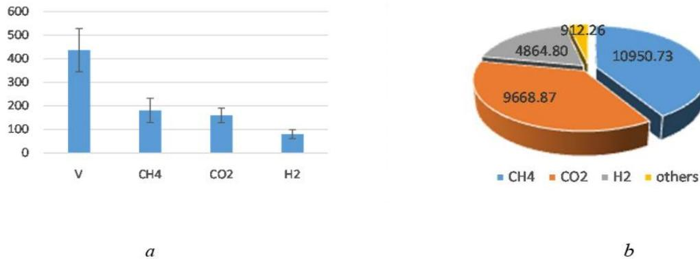
**Figure 4:** Biogas yield and composition for 14 days of co-anaerobic digestion in 2-stage system: a) The volume of 1gVS of biogas and its components and b) total biogas components yield from 60.49 gVS
